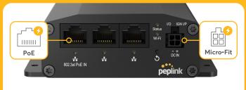
Power the device normally through Power over Ethernet for less cable management, or an industrial microfit connector for a secure and durable power option.
