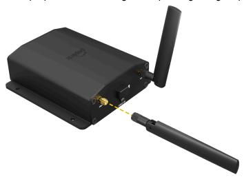
'If required, install Peplink's Mobility Antennas with an extension cable and position antenna to get a better signal strength.
