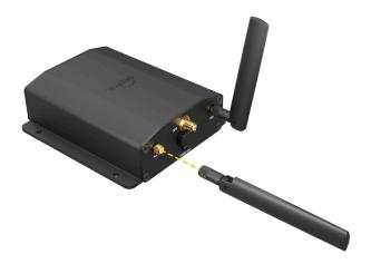
'If required, install Peplink's Mobility Antennas with an extension cable and position antenna to get a better signal strength.
